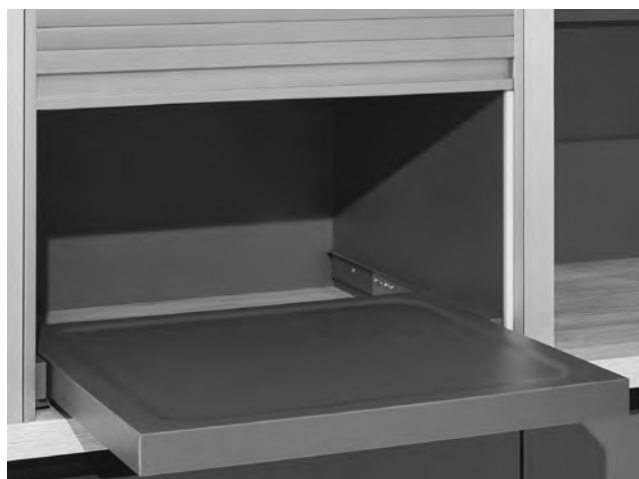
INTERNAL TABLAR WITH LOCKING DRAWER SLIDES ITAB-AJ60 FOR RETROFITTING IN DRESSER-ROLL-UP UNITS, 600 mm wide, laminate coated in Slate grey on both faces, polymer edge all around, with leak protection recess for liquids, Dimensions tablar shelf: H x W x D = 532 x 39 x 485 mm, Dimensions leak protection recess: H x W x D = 482 x 2.5 x 435 mm
